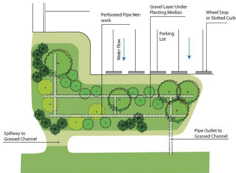
Raingarden example with underdrain
